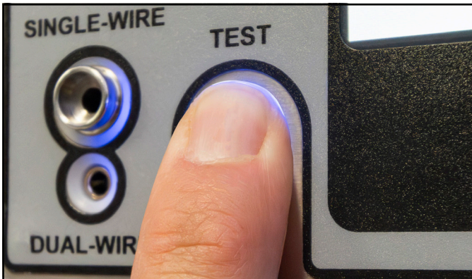
Figure 10. Bridging the test switch's contacts
