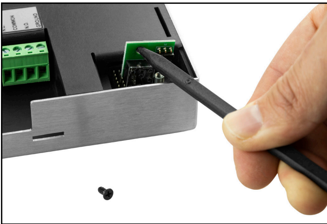
Figure 15. Lifting the used dual-wire wrist strap jack from the Combo Tester X3+
