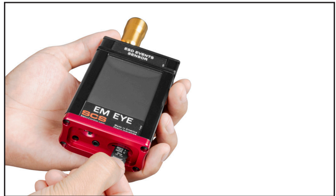
Figure 3. Inserting a microSD card
