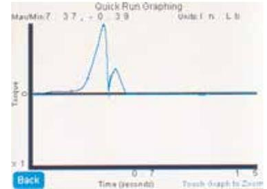
Resulting graph displays torque vs. time. Tap an area of the graph to zoom up to 4 times the size.
