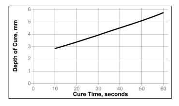
LED Flood Array 405nm, 100 mW/cm<sup>2</sup> , measured @ 405 nm
