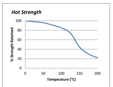
"Hot strength" shear strength tests performed on mild steel. Fully cured then conditioned to pull temperature for 30 minutes before testing. ES578 can withstand higher temperatures for brief periods (such as for paint baking and wave soldering processes) providing the joint is not unduly stressed. The minimum temperature the cured adhesive can be exposed to is -40°C (-40°F) depending on the materials being bonded.
