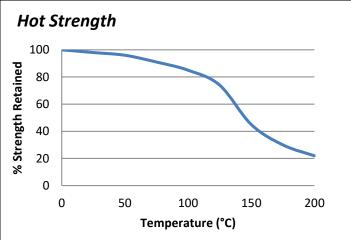
"Hot strength" shear strength tests performed on mild steel. Fully cured then conditioned to pull temperature for 30 minutes before testing.
