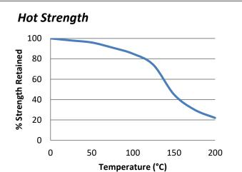
"Hot strength" shear strength tests performed on mild steel. Fully cured then conditioned to pull temperature for 30 minutes before testing. ES550 can withstand higher temperatures for brief periods (such as for paint baking and wave soldering processes) providing the joint is not unduly stressed.
