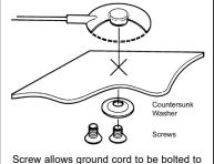
mat to keep cord from disconnecting. NOTE: Use a punch or Philips screw driver to create a hole in the mat.
