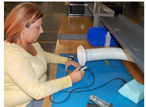
Two operators using the Floor Sentry Double unit to extract soldering fumes simultaneously.
