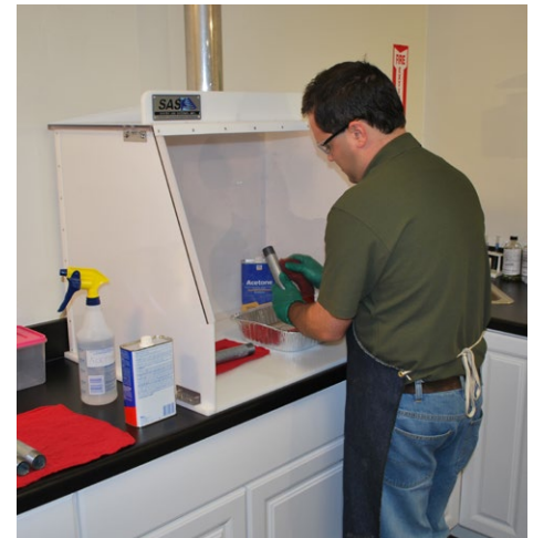
Ducted Fume Hoods provide useful fume extraction for various applications (30" pictured).
