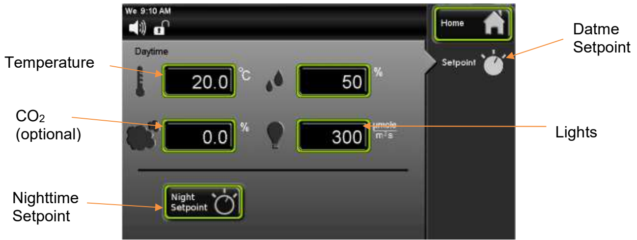
Day/Night setpoint screen for parameters, nighttime setpoint.
