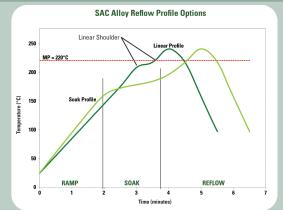
The stated profile recommendations apply to most Pb-free alloys in the SnAgCu (SAC) alloy system, including SAC305 (96.5Sn/3.0Ag/0.5Cu). This can be used as a general guideline in establishing a reflow profile when using **Indium10.1** Solder Paste. Deviations from these recommendations are acceptable, and may be necessary, based on specific process requirements, including board size, thickness, and density. Start with the linear profile, then move to the optional soak profile, if needed.
