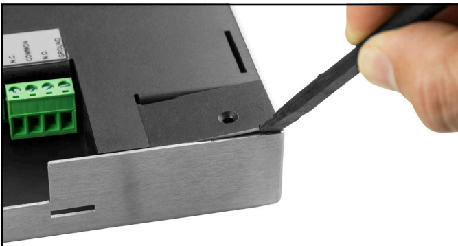
Figure 29. Opening the access cover
