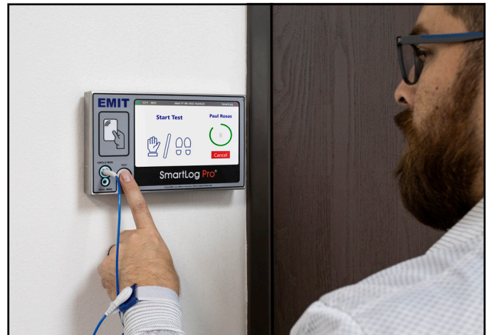
Figure 26. Performing a single-wire wrist strap test
