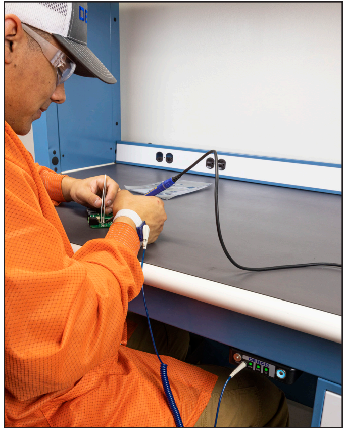
Figure 9. Using the Full-Time Continuous Monitor when mounted underneath a workbench tabletop
