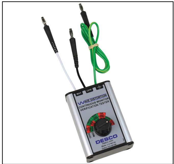
Figure 13. Desco 98221 Wave Distortion Monitor Verification Tester
