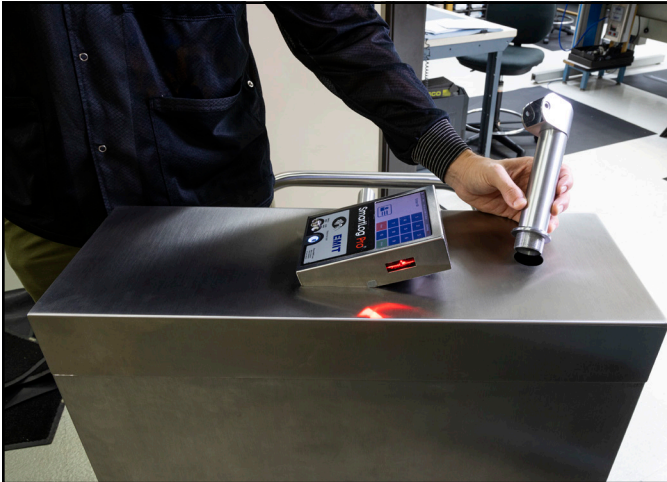
Figure 3. Inserting the mounting post into the hole in the turnstile's lid
