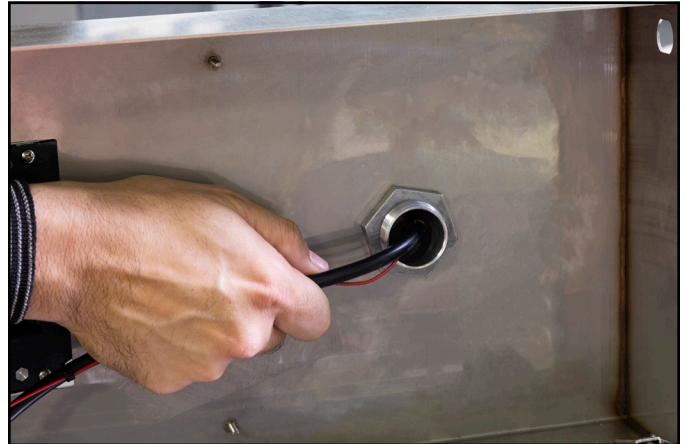
Figure 5. Feeding the wire harness from the Wiegand-to-USB Converter through the mounting post
