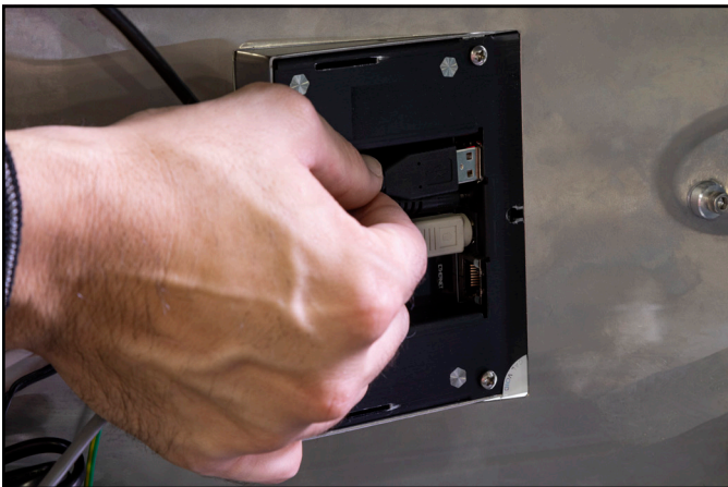
Figure 13. Connecting the USB cable to the SmartLog Pro®
