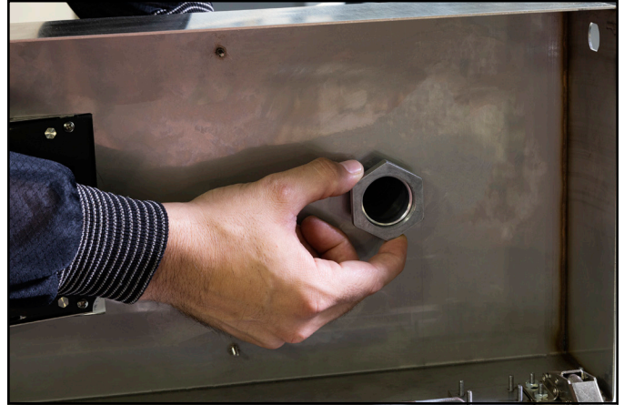
Figure 4. Using the nut to secure the mounting post onto the turnstile's lid
