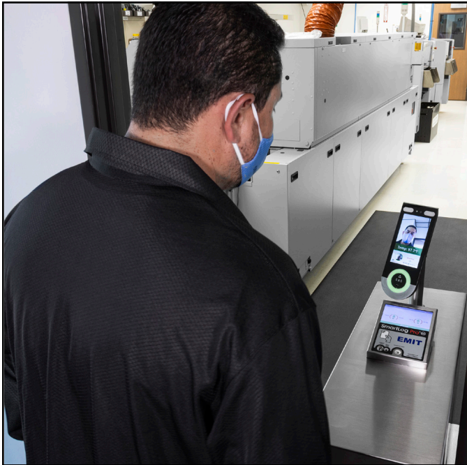
Figure 21. Using the Face Recognition Terminal to identify an operator and enforce the wearing of a face mask
