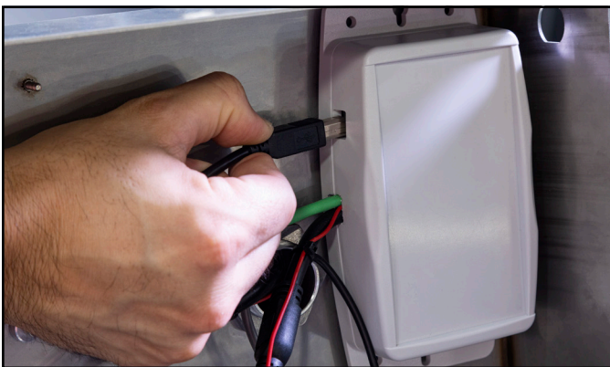
Figure 14. Connecting the USB cable to the Wiegand-to-USB Converter
