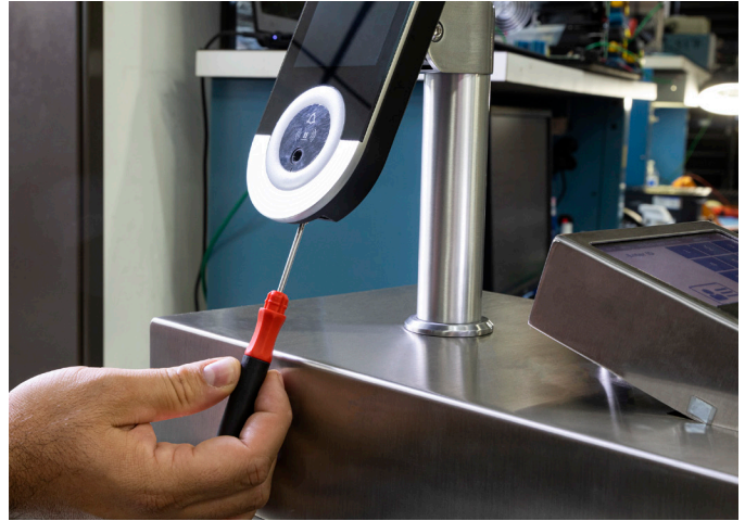
Figure 10. Securing the Face Recognition Terminal to the back plate
