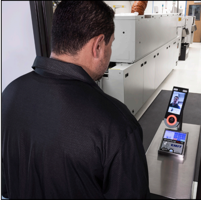
Figure 20. Using the Face Recognition Terminal to identify an operator
