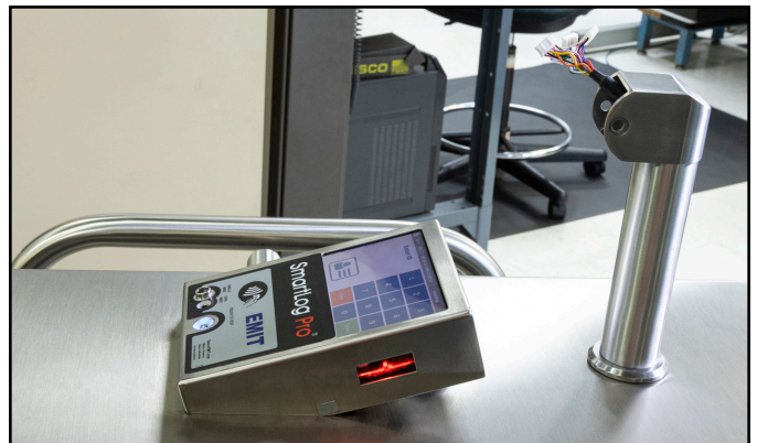
Figure 6. Routing the wire harness out the mounting post
