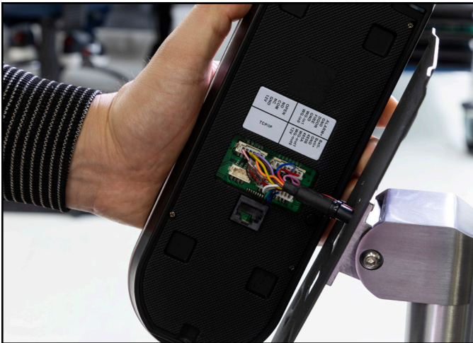
Figure 9. Connecting the wire harness to the Face Recognition Terminal
