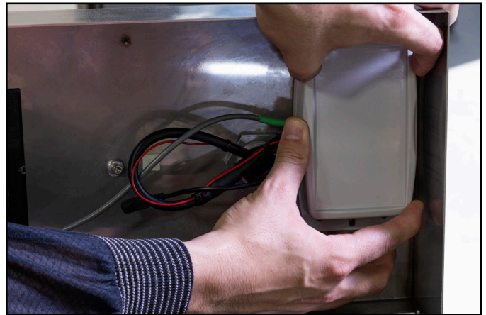
Figure 11. Mounting the Wiegand-to-USB Converter onto the turnstile's lid
