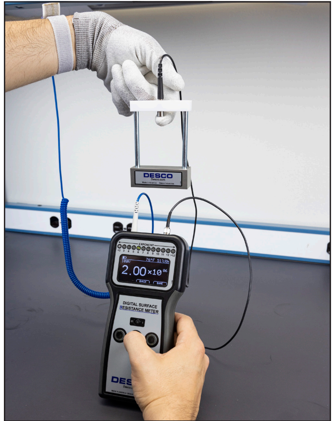
Figure 2. Using the Glove CAFE Test Electrode with the Desco 19290 Digital Surface Resistance Meter
